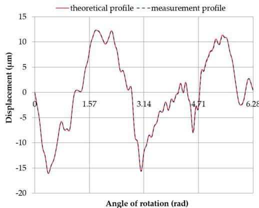
**Figure 24.** Measured and theoretical profiles (excluding harmonic component no. 1) obtained by superimposing the measured roundness profile of journal no. 5 onto the full eccentric movement profile of the center of the measured roundness profile.
