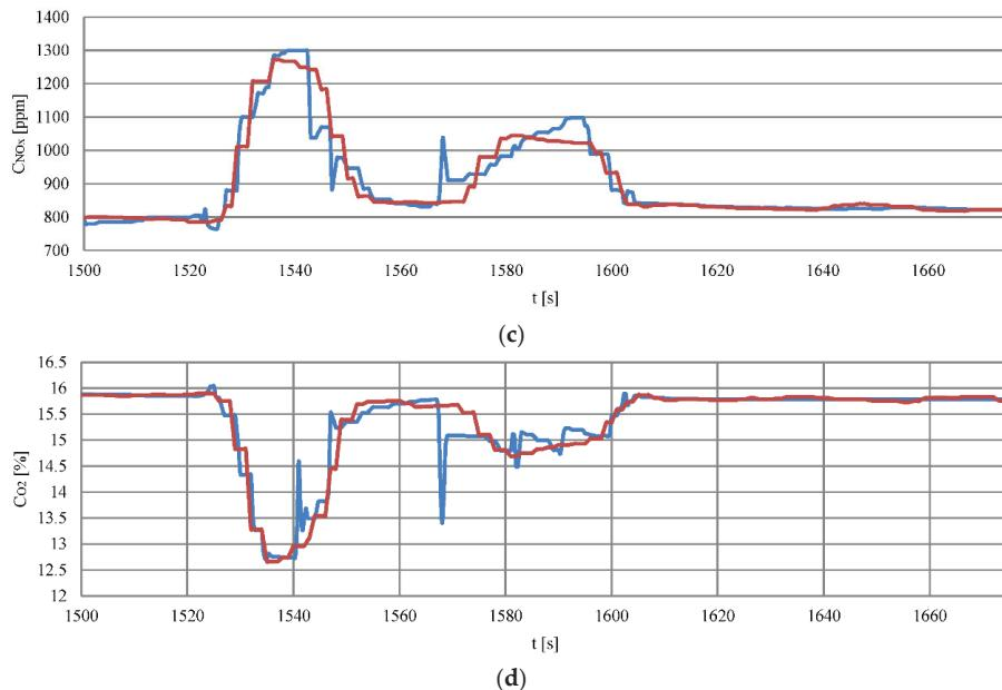
**Figure 12.** The courses of changes concentrations: (a) Carbon monoxide, (b) carbon dioxide, (c) nitrogen oxides, (d) oxygen during moving off maneuver as a function of time, red line—recorded data, blue line—data from the model.
