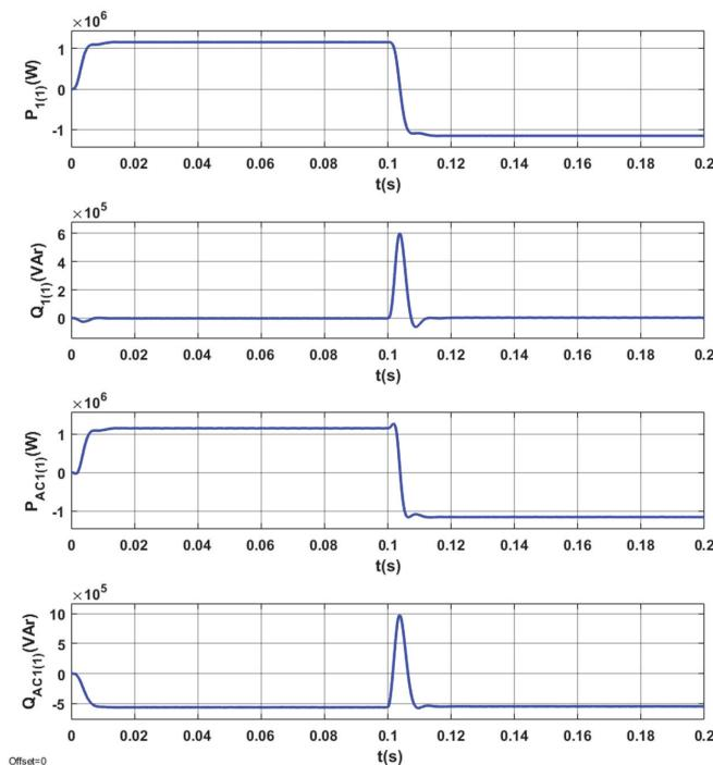
**Figure 13.** Energy processes  $P_{1(1)}$ ,  $Q_{1(1)}$ ,  $P_{AC1(1)}$ ,  $Q_{AC1(1)}$  in the optimized STS system, when switching AC\_1 from the operating mode corresponding to the active rectifier to the operating mode with the network inverter.
