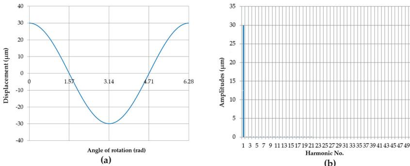
**Figure 18.** Eccentric movement profile of the center of the roundness profile being measured. The eccentricity was  $0.03 \text{ mm}$ , and the support did not limit the shaft displacement (a); discrete amplitude spectrum (b).**Table 5.** Amplitudes of the harmonic components for the eccentric movement of the center of the roundness profile being measured for eccentricity  $e = 0.03 \text{ mm}$  where the support does not limit the shaft displacement.
