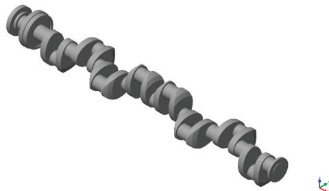
**Figure A1.** A 3D model of the crankshaft S-9285-3600-10-8-149-144-O-01.
