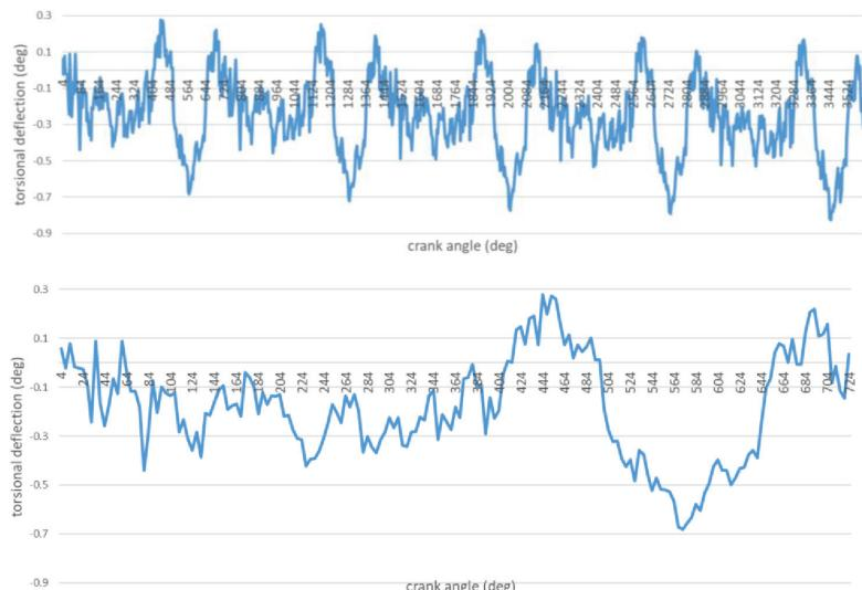
**Figure 6.** Torsional vibrations of the shaft as a function of the shaft rotation angle. DEU with a defect-free/healthy ship engine (ten turns and one cycle).
