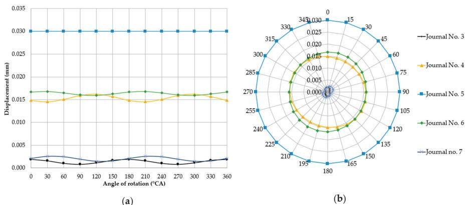
**Figure 7.** Changes in deflections measured in the vertical plane at individual main journals with the shaft rotated by 15° at a time and when one of the supports (of journal no. 5 counting from the timing gear end) is offset upwards by 0.03 mm relative to the others, shown in the charts in the (a) Cartesian and (b) polar coordinate systems.
