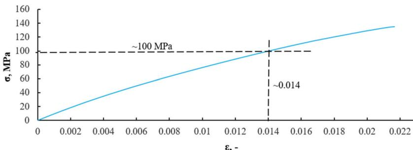
**Figure 10.** Determination of stress value on a composite without recyclate sample corresponding to strain  $\varepsilon = 0.014$  (90 s of time in Figure 9).
