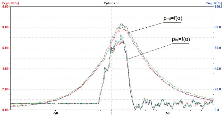
**Figure 5.** The diagram (screenshot of Unitest 2008) illustrates the  $p_{\text{cyl}} = f(\alpha)$  function with fuel injection characteristics of  $p_{\text{inj}} = f(\alpha)$  for a diesel–electric unit (DEU) with a defect-free/healthy ship engine loaded at 70% of MCR. Waveforms for cylinder: — No. 1, — No. 2, — No. 3.
