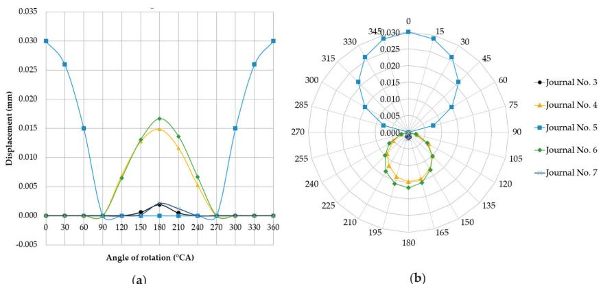
**Figure 10.** Changes in deflections measured in the vertical plane at individual main journals with the shaft changed by  $15^\circ$  at a time, and when one of the main journal axes (of journal no. 5 counting from the timing gear end) was offset eccentrically upwards by 0.03 mm relative to the others, shown in the (a) Cartesian and (b) polar coordinate systems.
