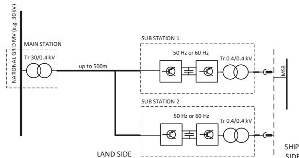
**Figure 2.** Selected topology of the STS system in accordance with the International Electrotechnical Commission (IEC)/International Organization for Standardization (ISO)/Institute of Electrical and Electronics Engineers (IEEE) standard.
