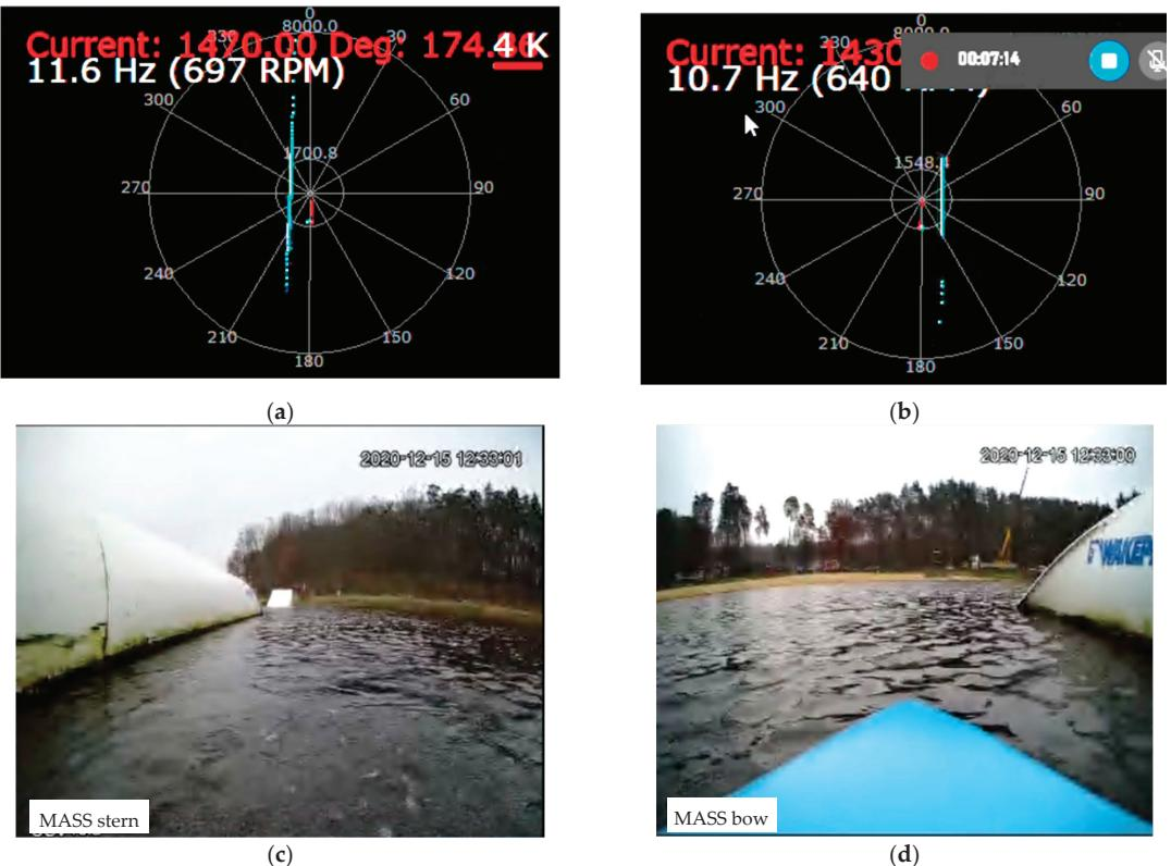
**Figure 15.** The model floating along a fixed obstacle (Pos. 1 from Figure 8)—snapshot from lidar and camera screens: (a) stern lidar image; (b) bow lidar image; (c) stern camera image; (d) bow camera image.
