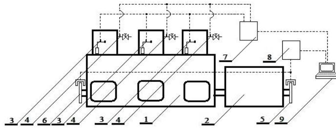
**Figure 2.** Block diagram of the test stand: 1—SULZER 3AL25/30 marine diesel engine; 2—Domel GD8 500-50/3 synchronous generator; 3—Kistler 4067E sensors for measuring pressure in the injection system; 4—Kistler 6353A24 sensors for measuring combustion pressure; 5,6—ETNP-10 laser heads tracking the movement of the perforated disc; 7—Unitest 2008 indicator; 8—ETNP-10 measuring and control block; 9—computer system for recording measurement data.
