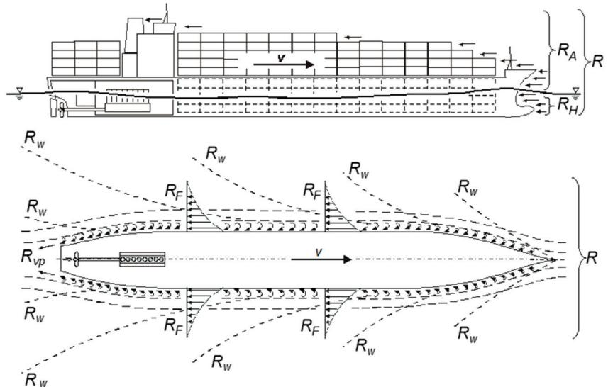
**Figure 3.** Distribution of the total hull resistance [13].
