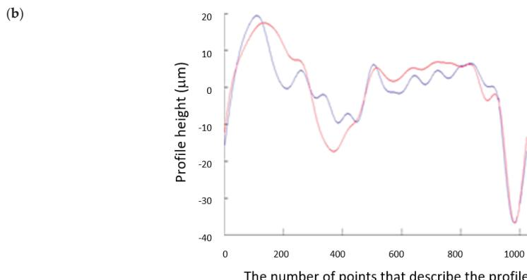
**Figure 6.** The measured (blue) and reference (red) profiles of journal No. 4 obtained for the controlled-reaction-force shaft support: (a) in polar coordinates; (b) in Cartesian coordinates.
