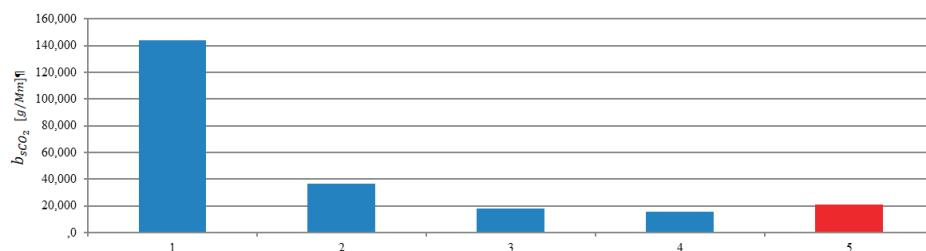
**Figure 19.** The ship's route carbon dioxide emissions during the stages: 1—Unberthing and hauling off maneuver, 2—moving off maneuver, 3—change of direction maneuver, 4—acceleration maneuver, 5—mean value of the ship's route emission.
