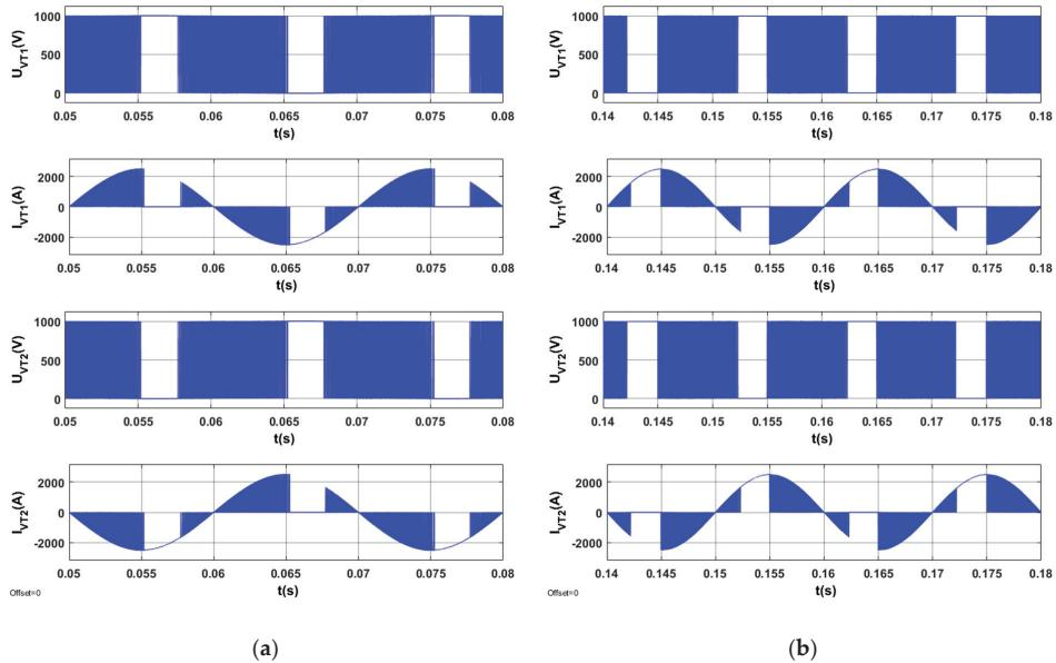
**Figure 16.** Voltages and currents on semiconductor elements of AC\_1's branch in the optimized STS system in the operating mode of an active rectifier **(a)** and in the operating mode of a network inverter **(b)**.
