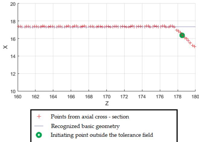
**Figure 9.** Chamfer detection based on axial cross-section.
