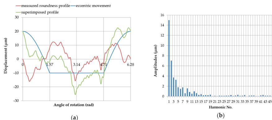
**Figure 21.** Profile obtained by superimposing the measured roundness profile of journal no. 5 on the eccentric movement profile of the center of the measured roundness profile with the supports set at the same height ( $x = 0 \text{ mm}$ ), with an eccentricity of the main journal  $e = 0.03 \text{ mm}$  (a); discrete amplitude spectrum of the superimposed profile (b).
