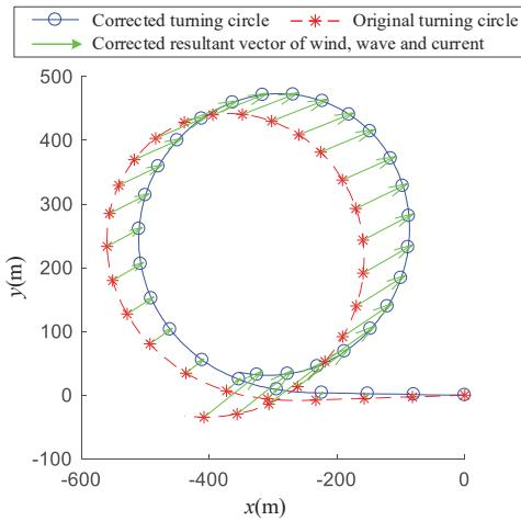
**Figure 9.** Correction of drift distance induced by the wind, waves and currents for  $+20^\circ$  turning circle test.
