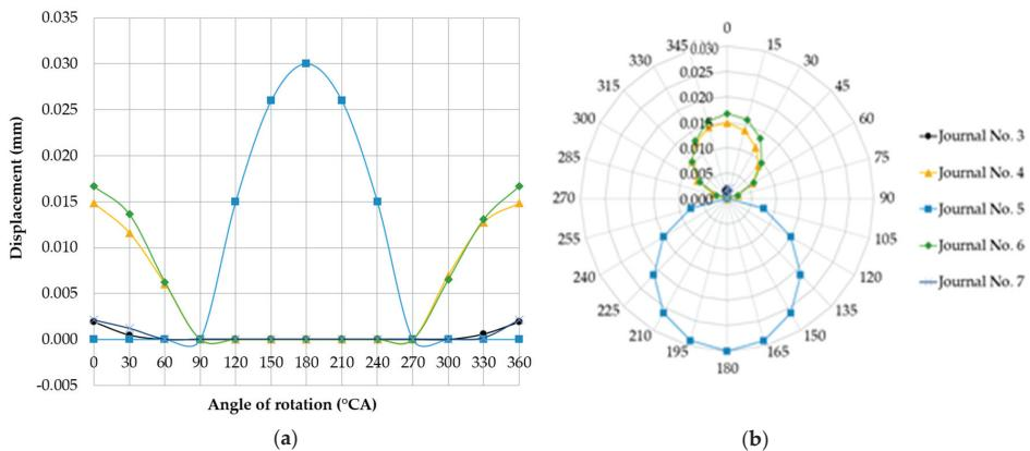
**Figure 11.** Changes in deflections measured in the vertical plane at individual main journals, when one of the main journal axes (no. 5 counting from the timing gear end) was offset eccentrically downwards by 0.03 mm relative to the others, shown in the (a) Cartesian and (b) polar coordinate systems.
