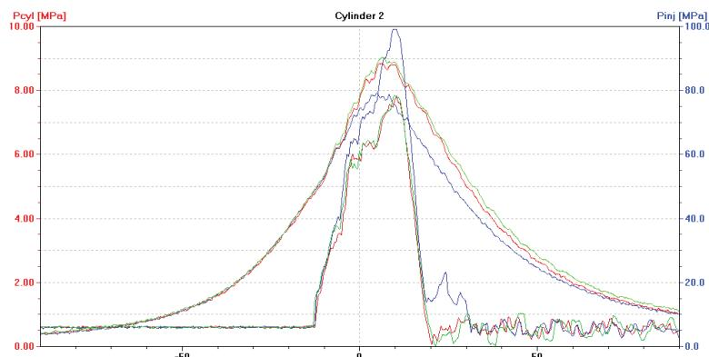
**Figure 10.** The diagram (screenshot of Unitest 2008) illustrates  $p_{cyl} = f(\alpha)$  with the fuel injection characteristics of  $p_{inj} = f(\alpha)$  for DEU with a defective ship engine-coked injector nozzle in the second cylinder, loaded at 70% MCR. Waveforms for cylinder: — No. 1, — No. 2, — No. 3.
