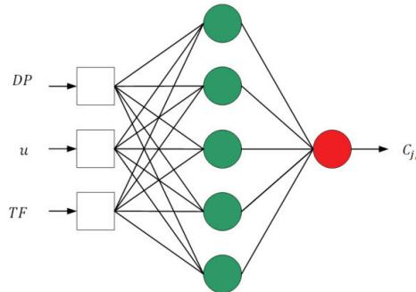
**Figure 6.** The neural network in configuration 3-5-1.  $DP$ —the fuel dose  $\left[\frac{g}{\text{rot.}}\right]$ ,  $u$ —the speed of a ship [knots],  $TF$ —the exhaust gases temperature  $[^\circ\text{C}]$ ,  $C_{j,i}$ —the concentration of exhaust gases components [ppm, %].
