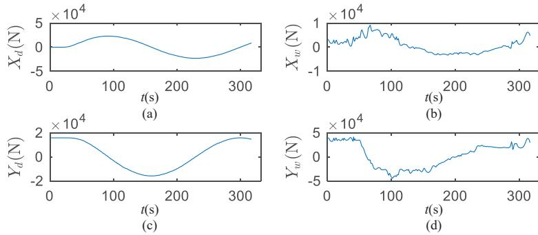
**Figure 6.** Wind load and wave drift force for  $+20^\circ$  turning circle test. (a) Surge force induced by wave; (b) surge load induced by wind; (c) sway force induced by wave; (d) sway load induced by wind.
