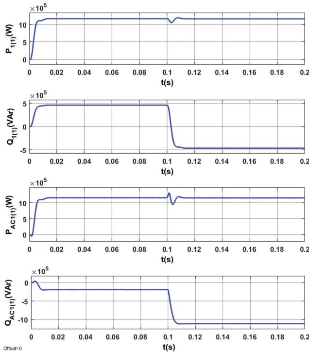
**Figure 17.** Energy processes  $P_{1(1)}$ ,  $Q_{1(1)}$ ,  $P_{AC1(1)}$ ,  $Q_{AC1(1)}$  in the STS system, taking into account the operating mode of the AC\_1 corresponding to the active rectifier ( $I_y = 2500$  A) and  $I_x$  changing from 1000 A to  $-1000$  A.
