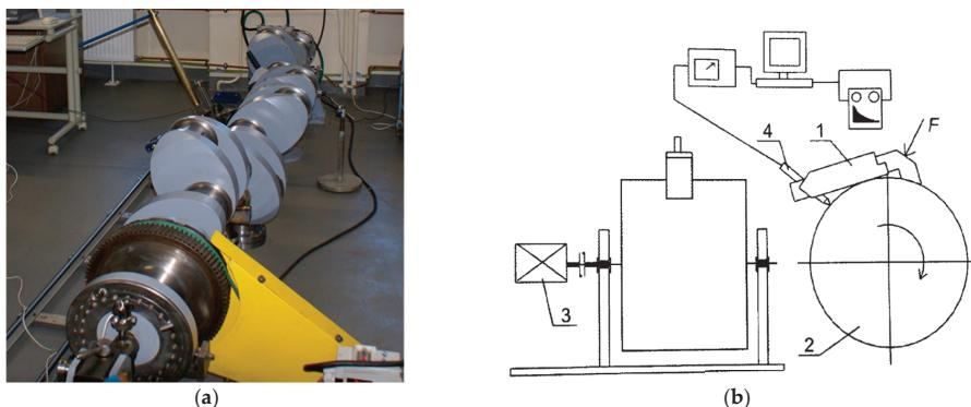
**Figure 5.** SAJD measurement system: (a) layout of the system; (b) measurement method [11]: 1—measuring head MUK 25-600, 2—shaft journal, 3—drive motor, 4—displacement sensor, F—measuring head pressing force.
