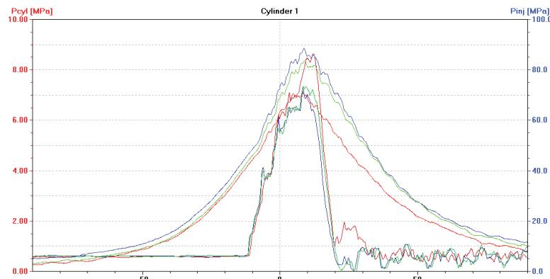
**Figure 9.** The diagram (screenshot of Unitest 2008) illustrates  $p_{cyl} = f(\alpha)$  with the fuel injection characteristics of  $p_{inj} = f(\alpha)$  for a DEU with a defective ship engine-coked injector nozzle in the first cylinder, loaded at 70% MCR. Waveforms for cylinder: — No. 1, — No. 2, — No. 3.
