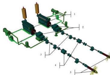
**Figure 2.** Visualization of the two-shaft main propulsion system with two controllable pitch propellers (CPP): 1—Main diesel engines, 2—reduction gears with auxiliary electric motors, 3—shaft lines, 4—CPP's hydraulic boxes, 5—CPP's.
