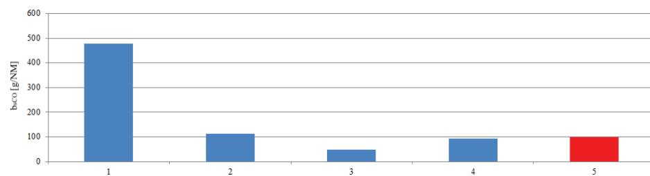
**Figure 18.** The ship's route carbon monoxide emissions during the stages: 1—Unberthing and hauling off maneuver, 2—moving off maneuver, 3—change of direction maneuver, 4—acceleration maneuver, 5—mean value of the ship's route emission.
