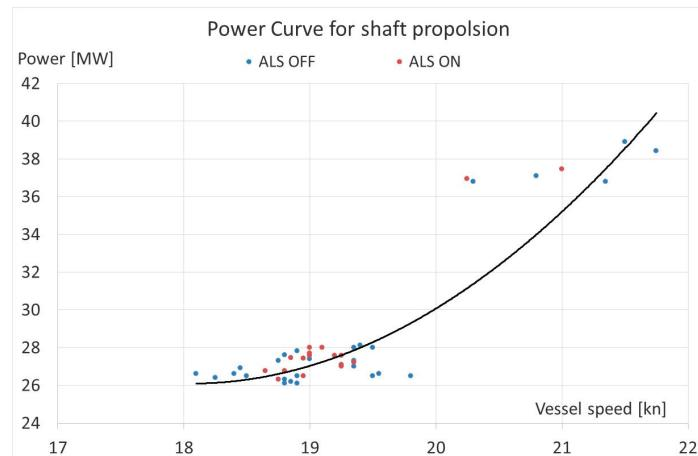
**Figure 11.** Average Shaft Power for given RPM against Speed from on cruise liner with diesel-electric propulsion.
