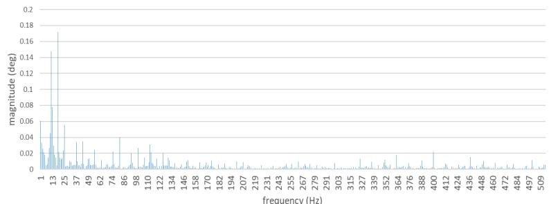
**Figure 7.** Full spectrum of torsional shaft vibrations. Diesel–electric unit with a defect-free ship engine.
