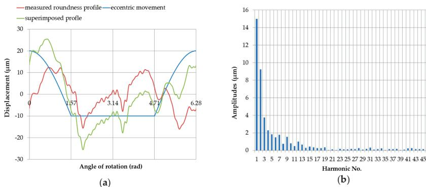
**Figure 22.** Profile obtained by superimposing the measured roundness profile of journal no. 5—rotated by  $60^\circ$  with respect to the reference profile—onto the profile of the eccentric movement of the center of the measured roundness profile, with the supports set at the same height ( $x = 0$  mm); with an eccentricity of the main journal  $e = 0.03$  mm (a); discrete amplitude spectrum of the superimposed profile (b).
