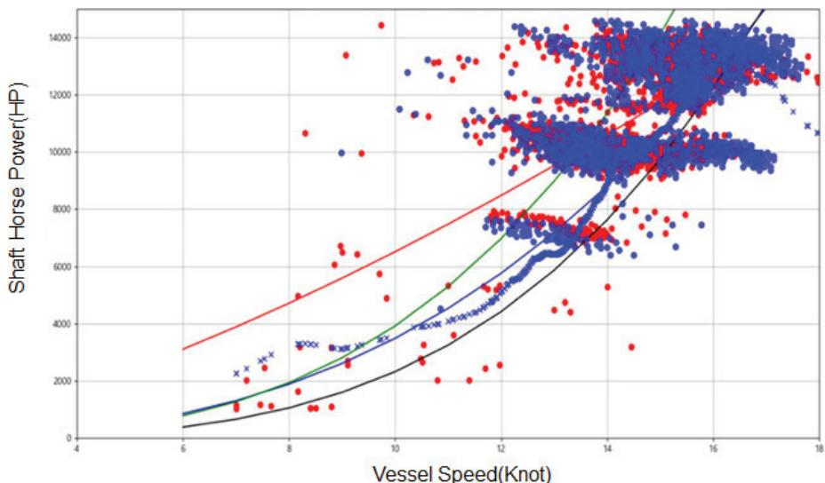
**Figure 4.** Comparison between predicted propulsion power vs. actual data.
