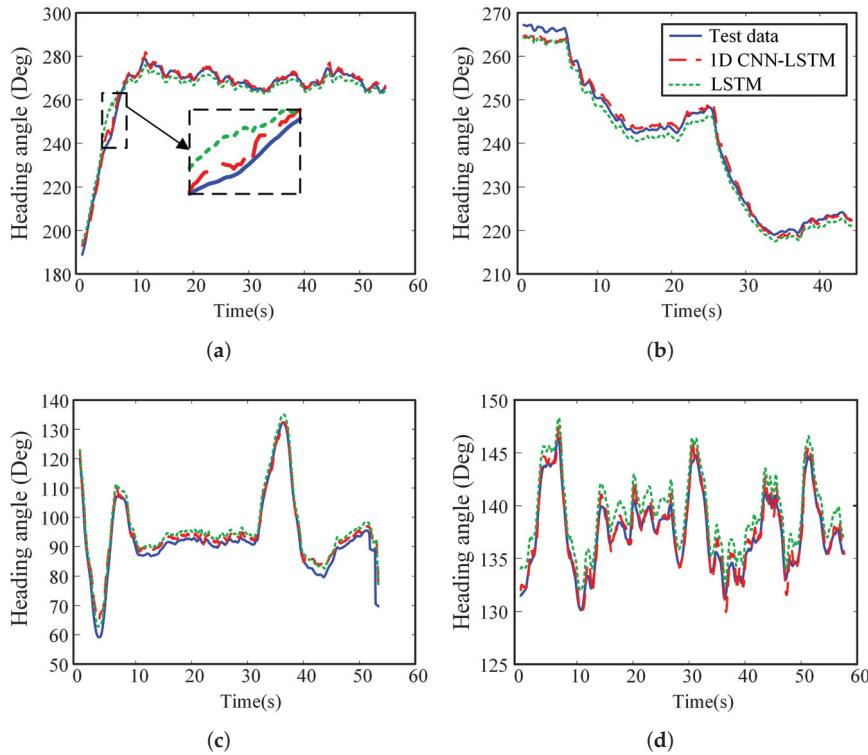
**Figure 7.** Comparison of the predict results and actual results by LSTM with CNN and LSTM without CNN at different sea level. (a) Level 1 sea condition. (b) Level 2 sea condition. (c) Level 3 sea condition. (d) Level 4 sea condition.
