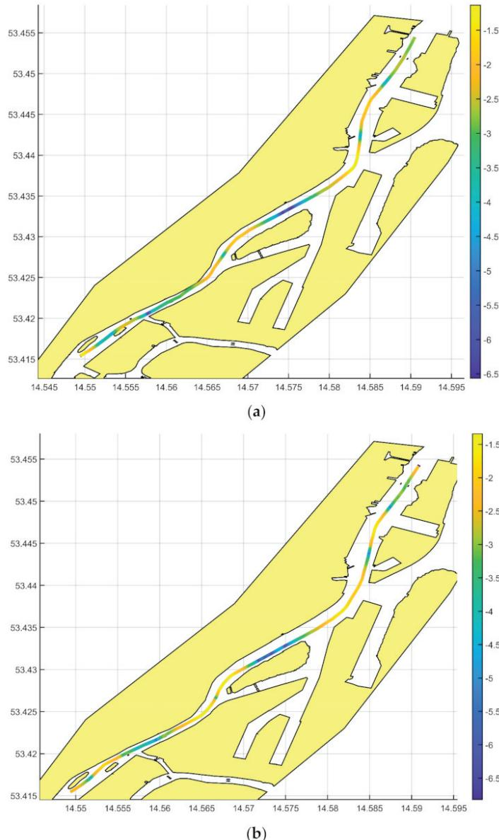
**Figure 5.** Impact of the curvature of the measurement profile on the recorded gravimetric signal. The spatial distribution of the correction is shown on the maps for the first line (a) and for the second line (b); a logarithmic scale is used.
