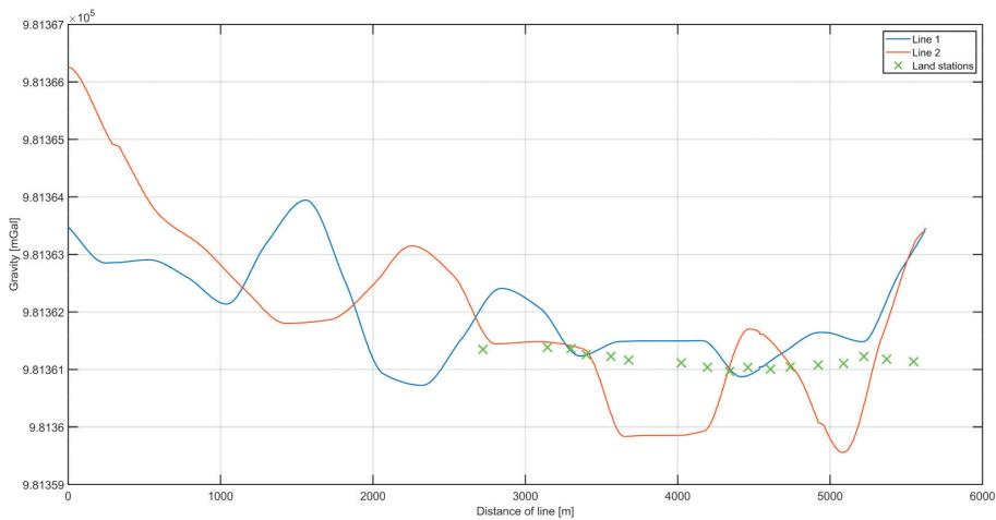
**Figure 8.** The superimposed values of gravitational acceleration on the two survey lines. In addition, land measurement points are marked, with the obtained values reduced to the height of the dynamic gravimeter.
