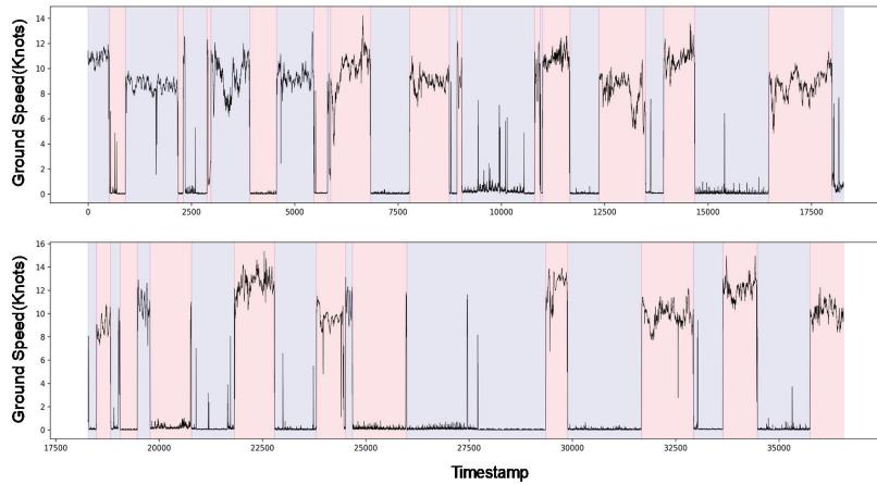
**Figure 3.** Time series of the vessel ground speed. Moreover, the windows-based change detection method is also applied to find operational regions among the dataset. The alternating color region indicates whether the vessel operates or not.
