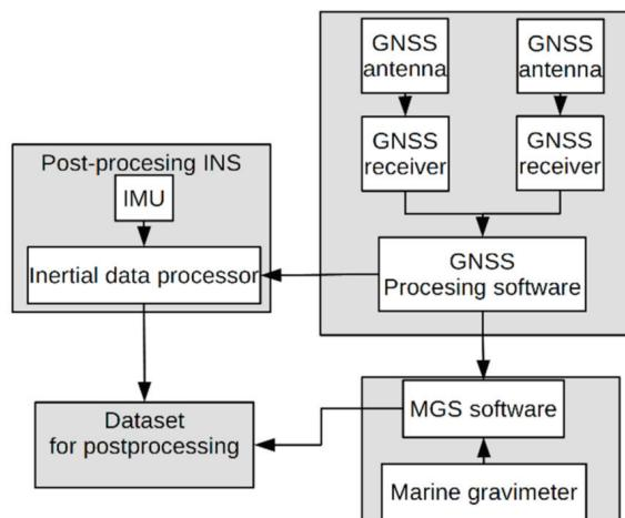
**Figure 1.** The scheme showing the flow of data during the measurement campaign. Abbreviations used: Global Navigation Satellite Systems (GNSS), Inertial Navigation System (INS), Inertial Measurement Unit (IMU), Marine Gravity System (MGS).
