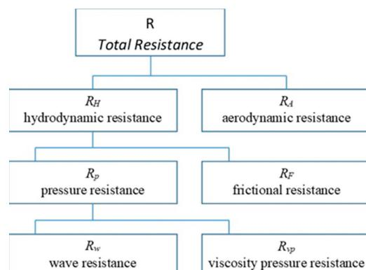
**Figure 2.** The total hull resistance structure [13].
