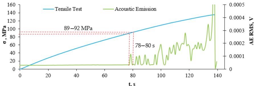
**Figure 11.** Graph of the value of the effective acoustic emission signal as a function of time, plotted on the stress-strain graph for a composite without recyclate.
