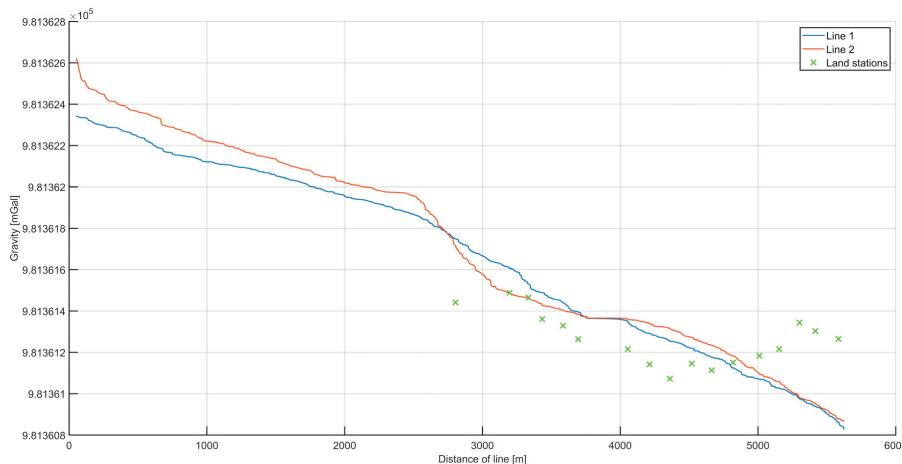
**Figure 12.** The superimposed values of gravitational acceleration on the two survey lines. In addition, land measurement points are marked, with the obtained values reduced to the height of the dynamic gravimeter. The data presented were processed as a result of the 20 Hz campaign.
