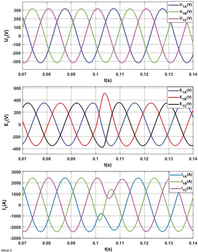
**Figure 15.** Electromagnetic processes in the optimized STS system, when switching the AC\_1 from the operating mode corresponding to the active rectifier to the operating mode with the network inverter.
