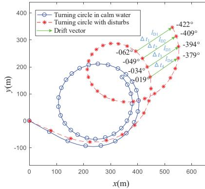
**Figure 1.** Traditional correction method of turning circle test.
