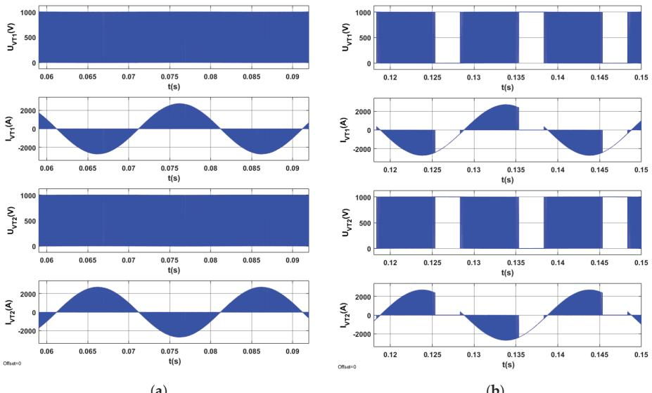
**Figure 20.** Voltages and currents on semiconductor elements of AC\_1's branch, which operates in the active rectifier mode in the STS system, (a)  $I_y = 2500$  A,  $I_x = 1000$  A, (b)  $I_y = -2500$  A,  $I_x = -1000$  A.
