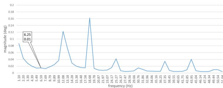
**Figure 8.** Mean value of torsional shaft vibration spectra. The diagram shows the 8th harmonic component only. Diesel–electric power unit with a defect-free ship engine.
