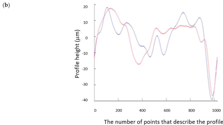
**Figure 5.** The measured (blue) and reference (red) profiles of journal No. 4, obtained for a shaft supported by a set of rigid V-blocks: (a) in the polar coordinate system; (b) in the Cartesian coordinate system.
