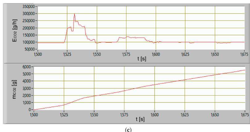
**Figure 14.** The courses of changes emissions intensity and emissions of exhaust gases components: (a) Nitrogen oxides, (b) carbon monoxide, (c) carbon dioxide during moving off maneuver as a function of time.
