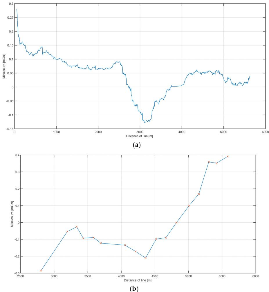
**Figure 13.** Misclosure analysis of repeated campaign: (a) The distribution of differences in the values of gravitational acceleration between the survey lines. (b) Distribution of differences between the gravity obtained on land and that measured on a survey line. The height differences have been reduced.
