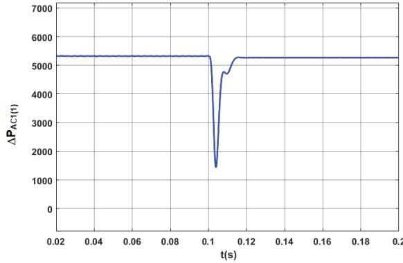
**Figure 14.** Power losses in the AC\_1 converter ( $\Delta P_{AC(1)}$ ) in the optimized STS system for the fundamental component, when switching the AC\_1 from the operating mode corresponding to the active rectifier to the operating mode with the network inverter.
