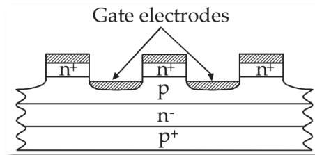
**Figure 2.** Cross section of a GTO showing the cathode islands and interdigititation with the gate (p-base).
