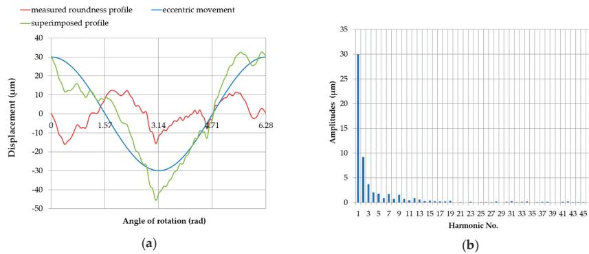
**Figure 20.** The profile obtained by superimposing the measured roundness profile of journal no. 5 on the full profile of the eccentric movement of the measured roundness profile center (a); discrete amplitude spectrum of the superimposed profile (b).
