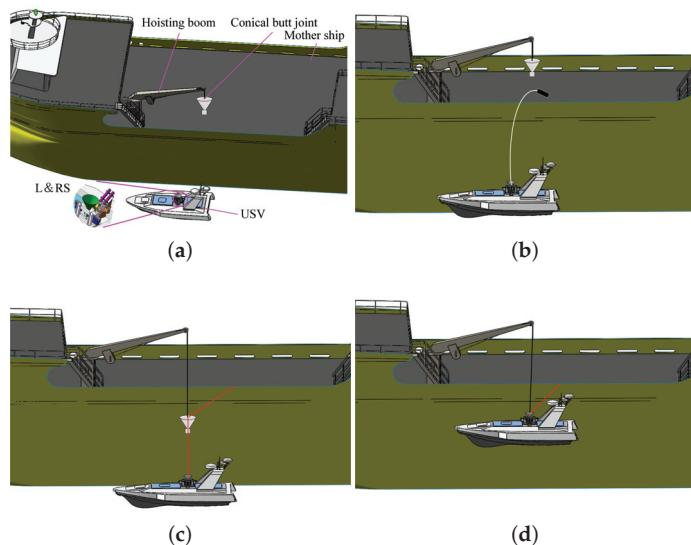
**Figure 2.** Operation process in recovering a USV. (a) Homing and aiming phase. (b) Launching phase. (c) Docking phase. (d) Lifting phase.
