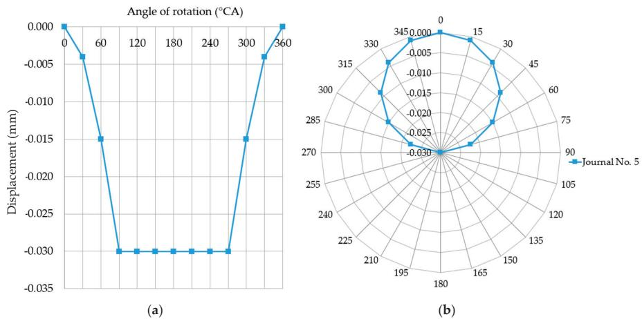
**Figure 13.** The journal displacements measured by the sensor for a full shaft rotation ( $0^\circ$ – $360^\circ$  angle) are recorded when the support maintaining a constant height restricts these displacements, as shown in the (a) Cartesian and (b) polar coordinate systems.
