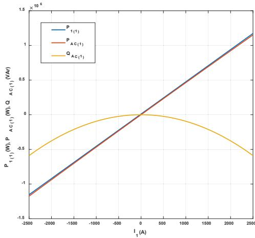
**Figure 9.** Energy characteristics of the optimized STS system.
