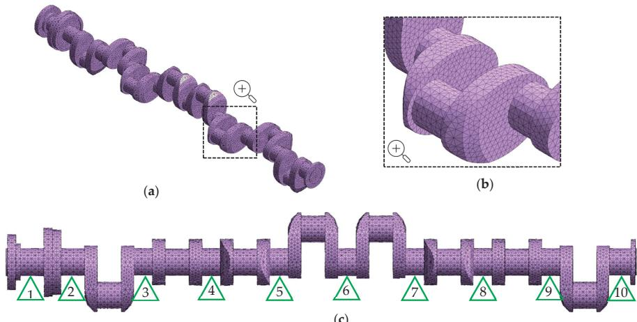
**Figure 4.** Finite element model of the analyzed shaft (a) isometric view; (b) mesh close-up; (c) main journals support.
