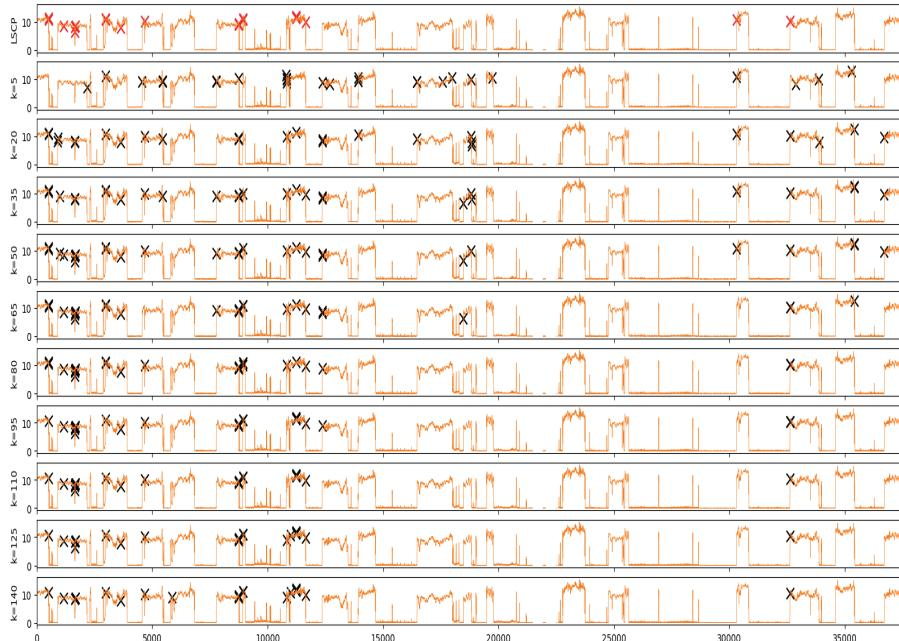
**Figure 7.** Comparison of anomaly detection results. The red mark indicates anomalies detected by the ensemble-based approach (LSCP), while the black mark indicates anomalies from individual detector Local Outlier Factor (LOF).
