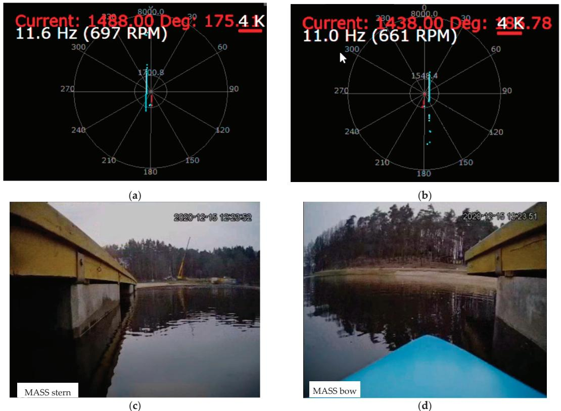
**Figure 11.** Unmooring maneuver from the platform (Pos. 1 from Figure 8)—snapshot from lidar and camera screens: (a) stern lidar image; (b) bow lidar image; (c) stern camera image; (d) bow camera image.
