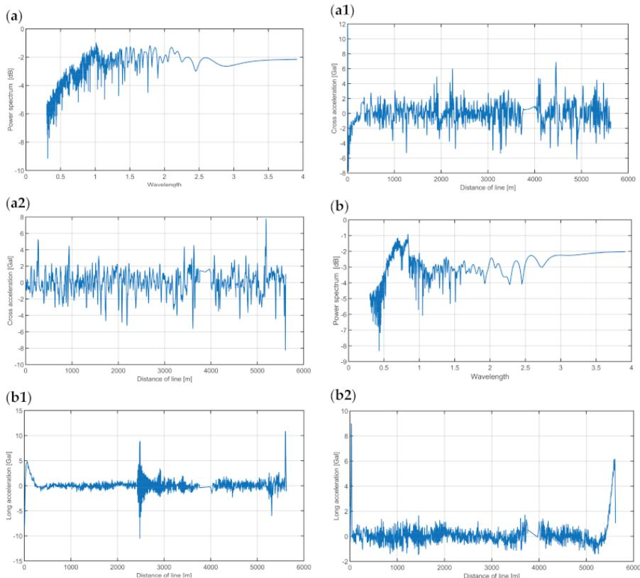
**Figure 6.** Signals from dilatometers installed in MGS-6. (a) Spectral power density for dilatometer signals for cross direction; (a1) values of cross accelerations of the first profile; (a2) values of cross accelerations of the second profile; (b) spectral power density for longitudinal direction; (b1) values of longitudinal accelerations for the first profile; (b2) values of longitudinal accelerations for the second profile.
