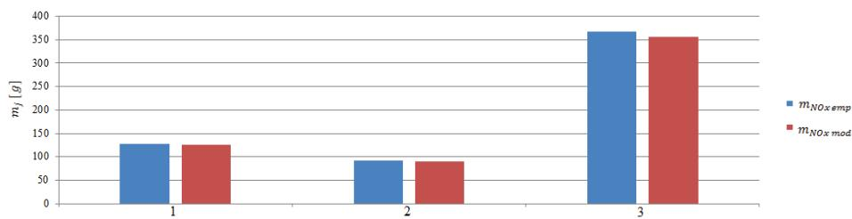
**Figure 17.** Nitrogen oxides emissions from model and empirical tests during the maneuvers: 1—Moving off, 2—change of direction, 3—acceleration.
