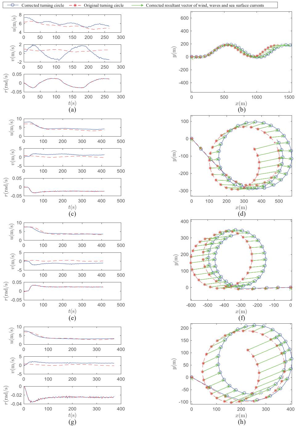
**Figure A4.** Correction result of track and velocities for test NO. 9–12. **(a)** Track of NO.9; **(b)** velocities of NO.9; **(c)** track of NO.10; **(d)** velocities of NO.10; **(e)** track of NO.11; **(f)** velocities of NO.11; **(g)** track of NO.12; **(h)** velocities of NO.12.
