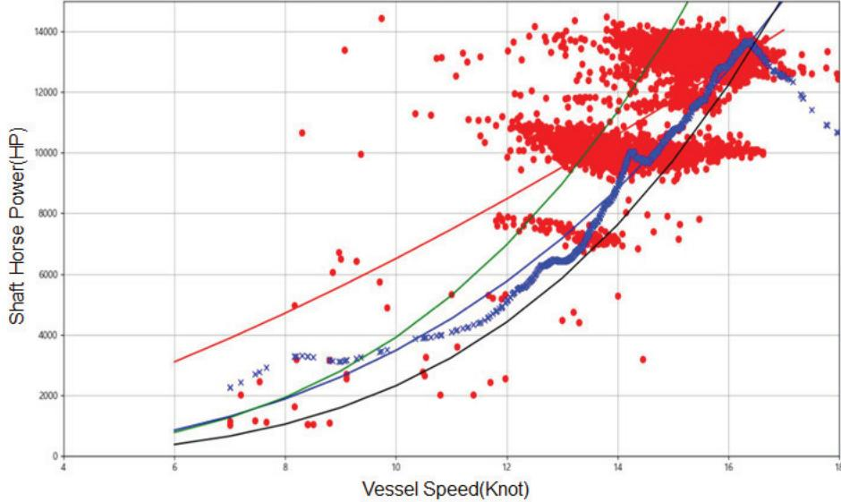
**Figure 5.** Predicted propulsion power without external effect.
