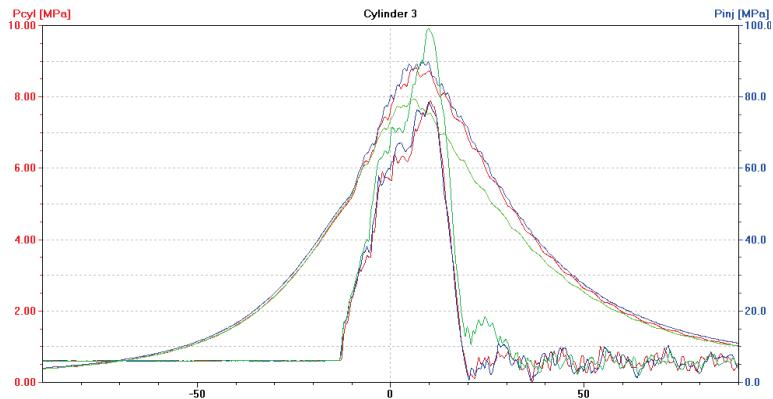
**Figure 11.** The diagram (screenshot of Unitest 2008) illustrates  $p_{\text{cyl}} = f(\alpha)$  with the fuel injection characteristics of  $p_{\text{inj}} = f(\alpha)$  for DEU with a defective ship engine-coked injector nozzle in the third cylinder, loaded at 70% MCR. Waveforms for cylinder: — No. 1, — No. 2, — No. 3.
