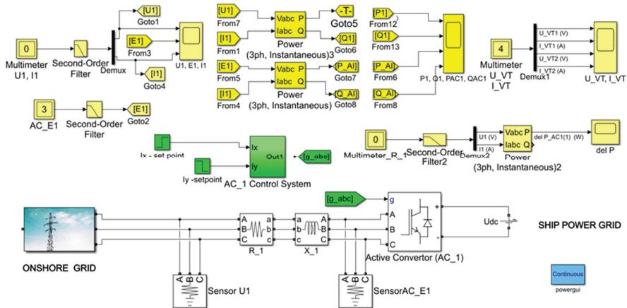
Figure 12. Simulation model of STS system.
