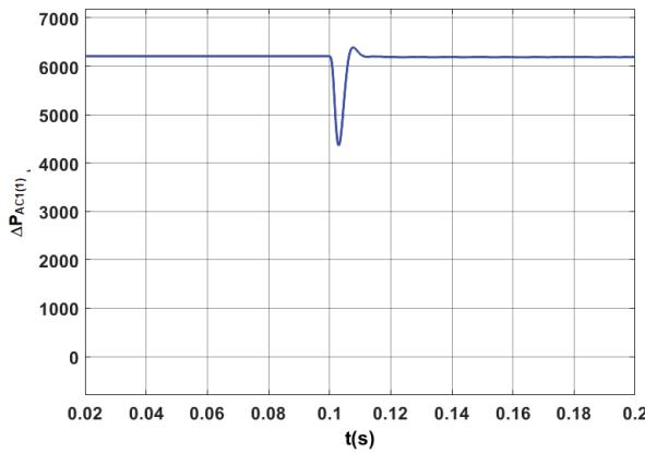
**Figure 18.** Power losses for the fundamental component in the STS system, taking into account the operating mode of the AC\_1 corresponding to the active rectifier ( $I_y = 2500$  A) and  $I_x$  changing from 1000 A to  $-1000$  A.
