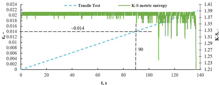
**Figure 9.** A metric entropy diagram applied on a strain diagram in the function of time, for a sample of composite without recyclate.
