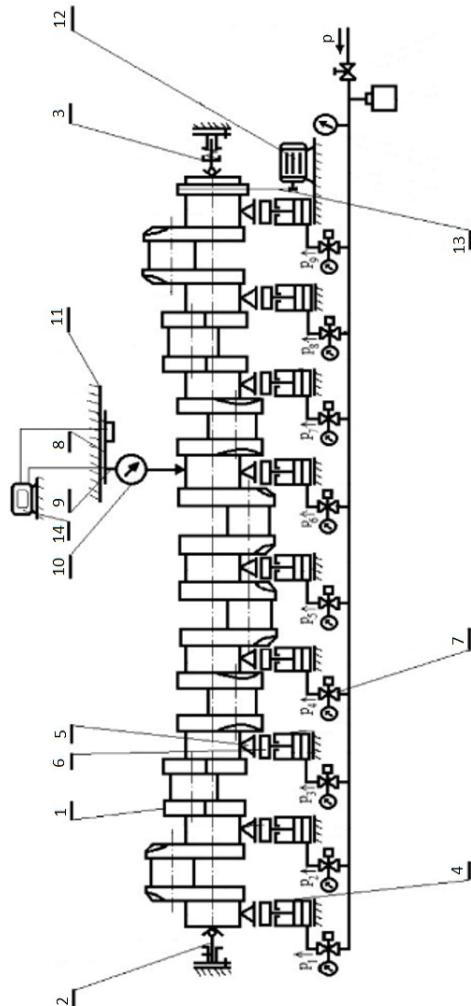
**Figure 1.** A diagram of the most essential components of the measuring system [6]: (1) crankshaft; (2,3) fixing centers; (4) support with pneumatic actuator; (5) V-block head; (6) force sensor; (7) current-controlled precision valve; (8) trolley; (9) tripod; (10) surface geometry sensor; (11) slide; (12) electric motor; (13) belt transmission; (14) PC with software.
