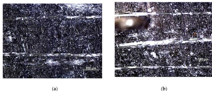
**Figure 7.** Composite structures: (a) without recyclate, (b) 10% of recyclate, magnification  $\times 100$ .
