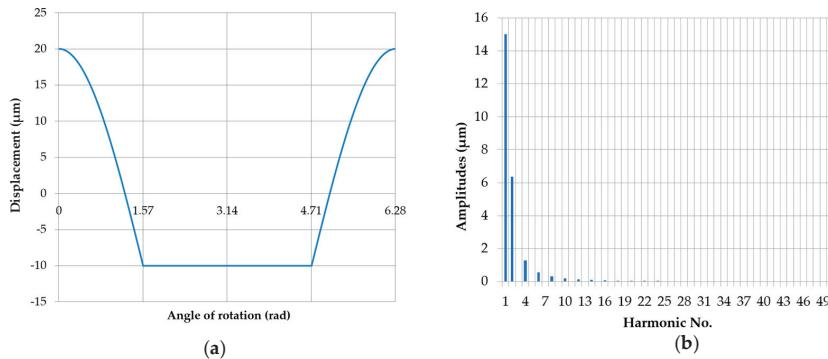
**Figure 19.** Eccentric movement profile of the center of the roundness profile being measured when the supports were set at the same height ( $x = 0$  mm), with an eccentricity of the main journal  $e = 0.03$  mm (a); discrete amplitude spectrum (b).
