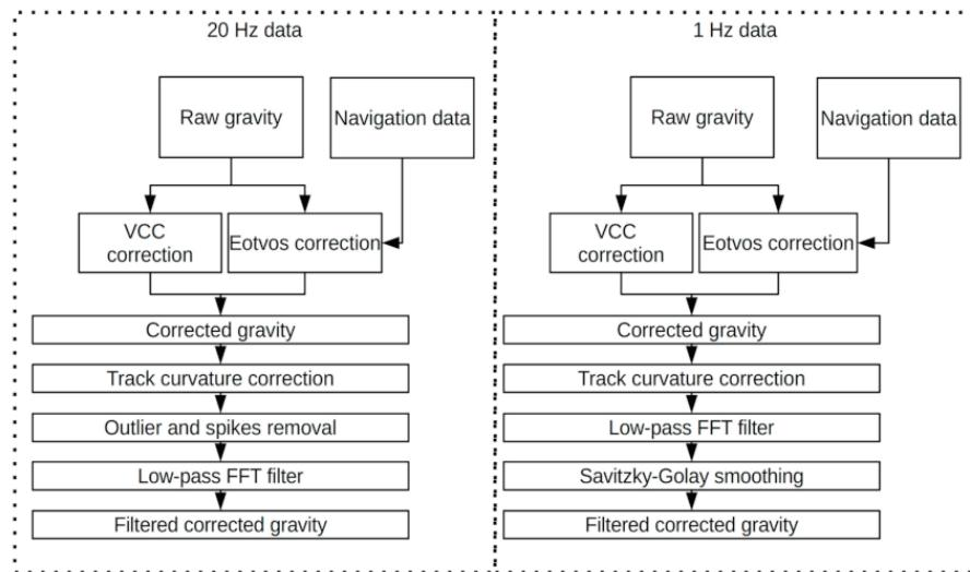
**Figure 7.** The block scheme showing the data processing routes for 20 Hz and 1 Hz gravimetric data. The FFT refers to Fast Fourier transform.
