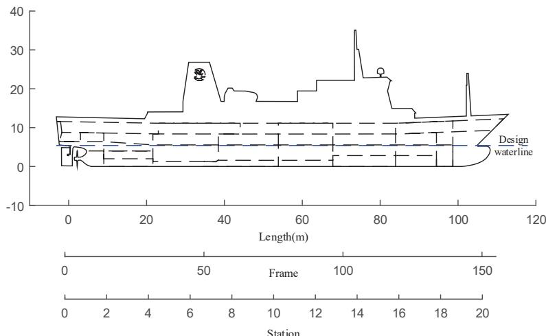
**Figure 3.** A general arrangement of Yukun motor vessel [29,30] (the figure permission has been achieved from Dalian Maritime University).
