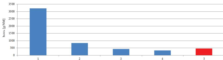
**Figure 20.** The ship's route nitrogen oxides emissions during the stages: 1—Unberthing and hauling off maneuver, 2—moving off maneuver, 3—change of direction maneuver, 4—acceleration maneuver, 5—mean value of the ship's route emission.
