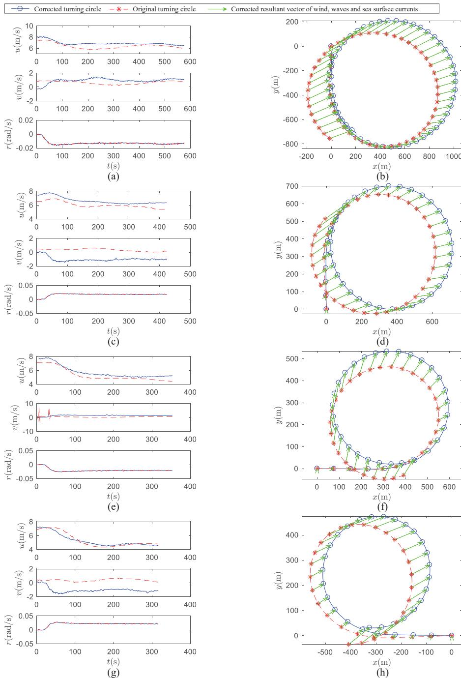
**Figure A2.** Correction result of track and velocities for test NO. 1–4. **(a)** Track of NO.1; **(b)** velocities of NO.1; **(c)** track of NO.2; **(d)** velocities of NO.2; **(e)** track of NO.3; **(f)** velocities of NO.3; **(g)** track of NO.4; **(h)** velocities of NO.4.
