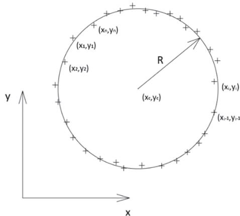
**Figure 6.** Approximation of the circular cross-section.
