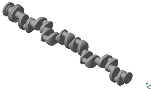
**Figure A2.** A 3D model of the crankshaft S-8658-3600-10-8-149-114-O-02.
