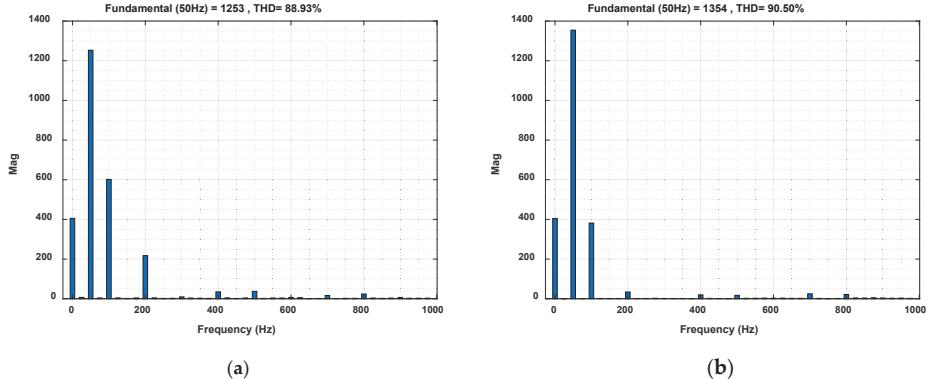
**Figure 21.** Current spectrum in the semiconductor element of the AC\_1 converter operating in the active rectifier mode with the optimized STS system (a) and  $I_y = 2500$  A,  $I_x = 1000$  A (b) for two of the 10 cycles of the selected current signal  $I_{VT1}$ .
