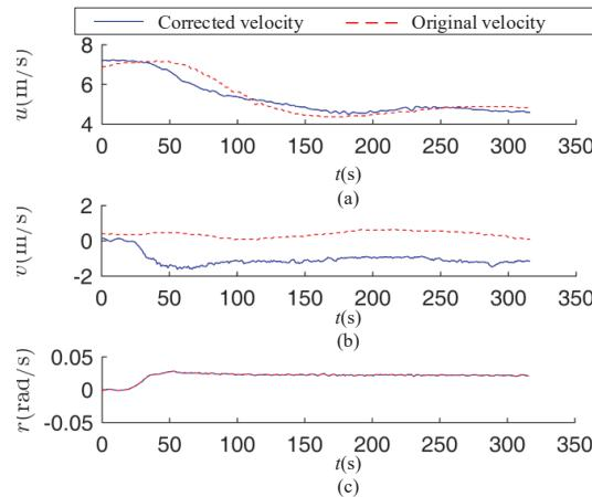
**Figure 10.** Correction of ECEF reference frame velocities for  $+20^\circ$  turning circle test. (a) Ship surge velocity; (b) ship sway velocity; (c) ship yaw velocity.
