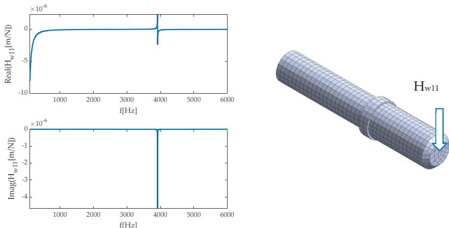
**Figure 12.** An example of FRF for the workpiece.
