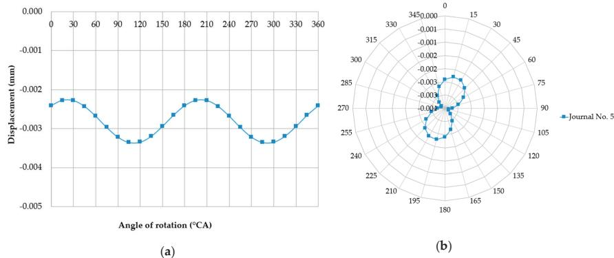
**Figure 9.** Changes in deflections measured in the vertical plane at individual main journals with the shaft rotated by  $15^\circ$  at a time and when one of the supports (of journal no. 5 counting from the timing gear end) was offset downwards by 0.03 mm relative to the others, in the (a) Cartesian and (b) polar coordinate systems.
