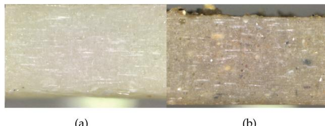
**Figure 1.** Cross-sections of composite materials with recyclate content of 1.2 mm granulation and percentage content: (a) 0%, (b) 10%, magnification  $\times 3$  (confocal microscope).
