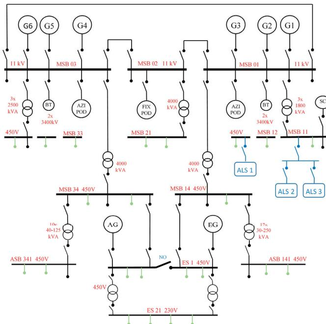
**Figure 8.** An example of simplified diagram of power distribution on a passenger ship with diesel-electric propulsion system.
