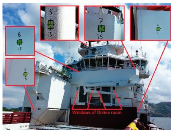
**Figure 3.** Common control points marked on the vessel.
