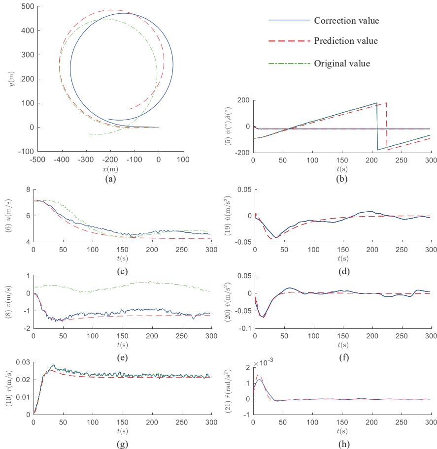
**Figure 11.** Prediction for +20° turning circle test. (a) Ship track; (b) ship heading angle and rudder angle; (c) surge velocity; (d) surge acceleration; (e) sway velocity; (f) sway acceleration; (g) yaw velocity; (h) yaw acceleration.
