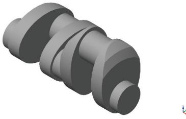
Figure A12. A 3D model of the crankshaft S-1977-0740-3-2-149-144-O-12.
