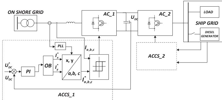
Figure 11. Block diagram of the STS system.
