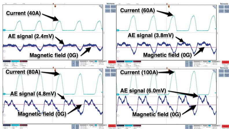
**Figure 9.** The chosen waveforms of raw AE signals (blue) detected by WS $\alpha$  transducer placed on the anode plate of conducting different currents (rectifying mode) GTO. Current and magnetic field waveforms placed for reference.
