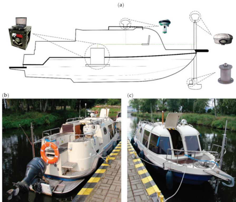
**Figure 2.** (a) Locations of the sensors on the research vessel, from left to right: MGS-6, GS 15, R8 and IMU-10. (b) The research vessel during preparation for the campaign: view from stern; (c) view from bow.
