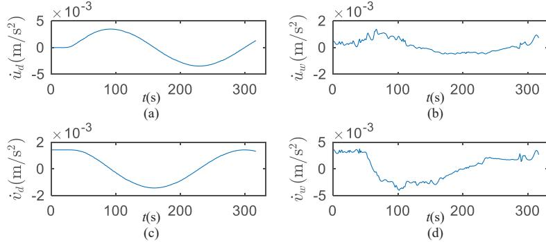
**Figure 7.** Wind- and wave-induced accelerations of  $+20^\circ$  turning circle test. (a) Surge acceleration induced by wave; (b) surge acceleration induced by wind; (c) sway acceleration induced by wave; (d) sway acceleration induced by wind.
