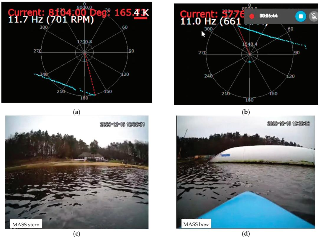
**Figure 13.** The model is floating towards the obstacle (Pos. 2 from Figure 8)—snapshot from lidar and camera screens: (a) stern lidar image; (b) bow lidar image; (c) stern camera image; (d) bow camera image.
