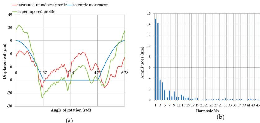
**Figure 23.** Profile obtained by superimposing the measured roundness profile of journal no. 5 (green)—rotated by  $90^\circ$  with respect to the reference profile—onto the eccentric movement profile of the center of the measured roundness profile (blue), with the supports set at the same height ( $x = 0$  mm) (a); discrete amplitude spectrum of the superimposed profile (b).
