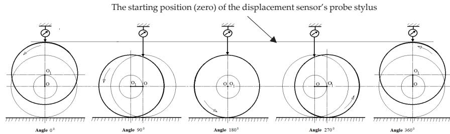
**Figure 12.** Supplementary diagram of the successive stages of shaft deflection caused by its eccentricity with respect to the axis of rotation of the measuring system when the support retains its fixed height.
