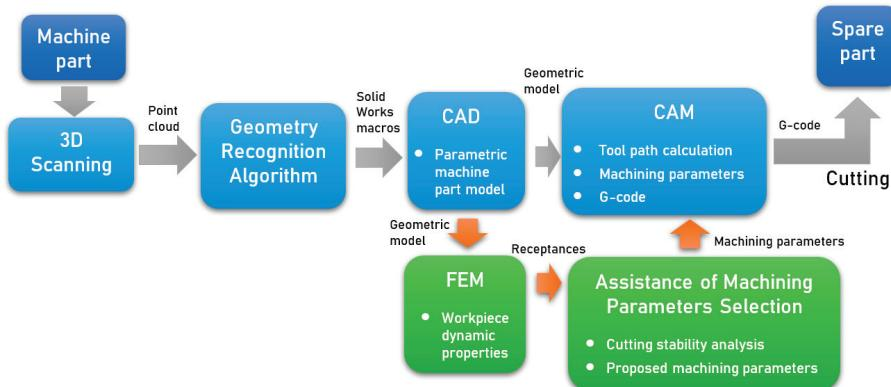
**Figure 1.** Block diagram showing the system concept.
