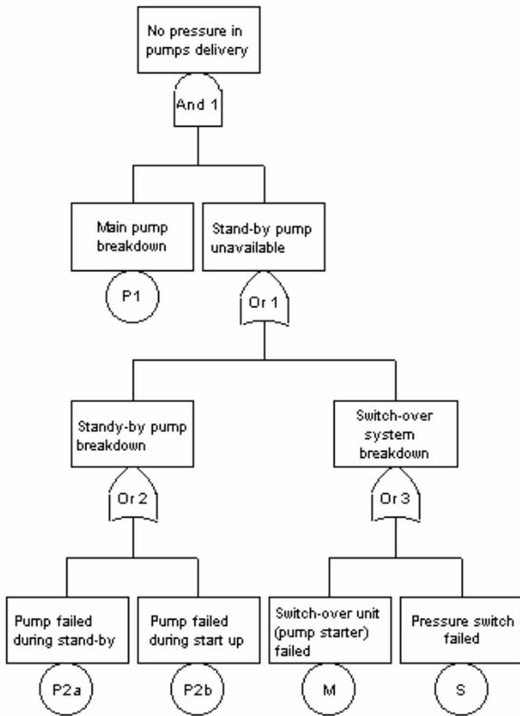
Fig. 4. Fault tree for real redundant pumps unit
