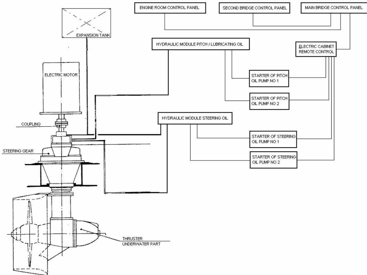
Fig. 1. Main components of example azimuth thruster system
