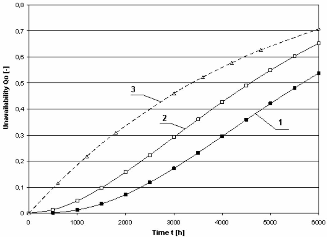
Fig. 4. Estimated unavailability  $Q_o(t)$  of injectors and whole system calculated with use of ERAC algorithm:
