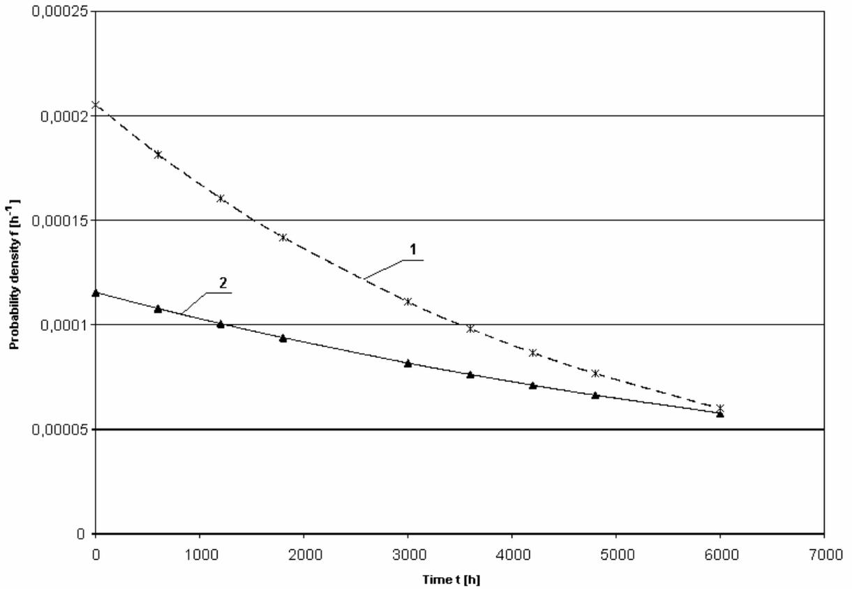
Fig. 3. Estimated probability density function  $f(t)$  of injectors: 1- real working time; 2 – calendar time
