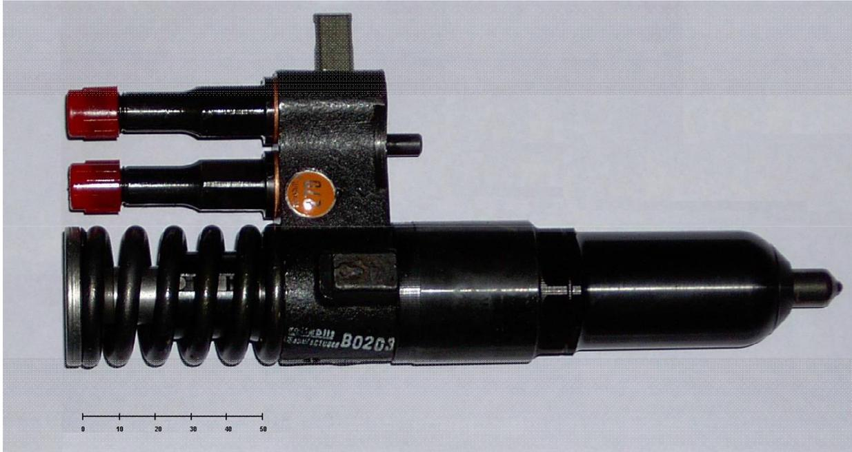
Fig. 1. View of Detroit Diesel 149 engine injector
