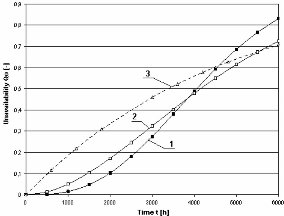
Fig. 5. Estimated unavailability  $Q_o(t)$  of injectors and whole system calculated with use of UBA method: 1 – fuel system – the engine rooms connected; 2– fuel system – the engine rooms divided; 3 – injectors.
