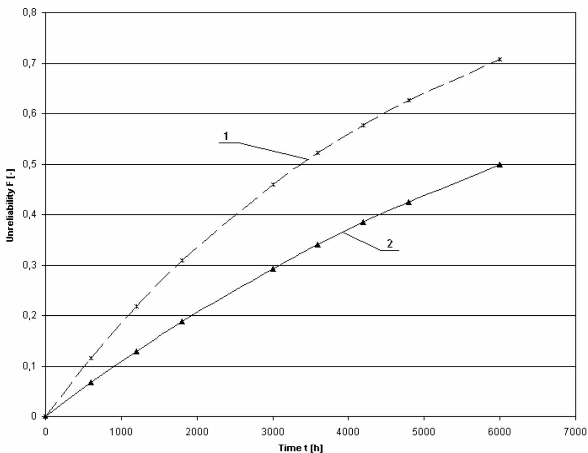
Fig. 2. Estimated unreliability function  $F(t)$  of injectors: 1- real working time; 2 – calendar time
