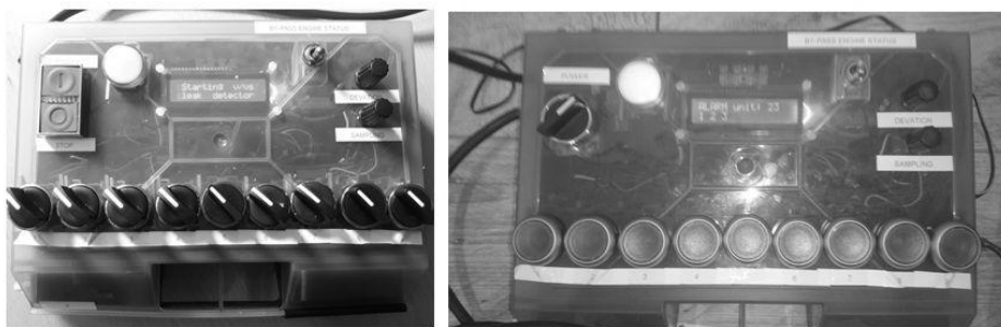
Fig. 6. Two versions of the front panel of the leak detector for starting valves
