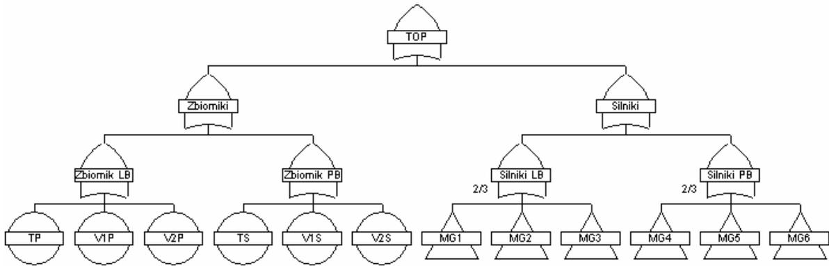
Fig. 7. A fault tree for the fuel system of the main generating set engines – valves separating power plants are closed
