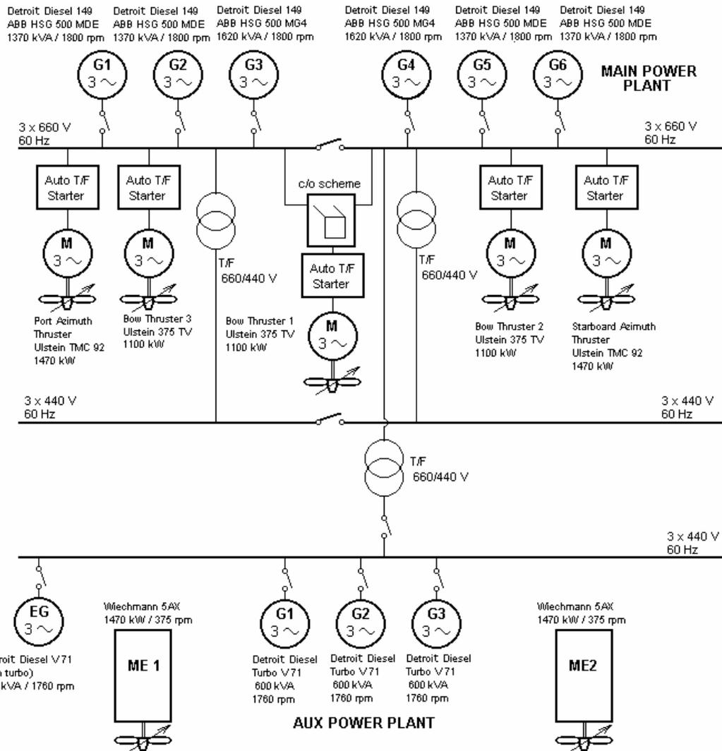
Fig. 2. The power-propulsion system of offshore vessel
