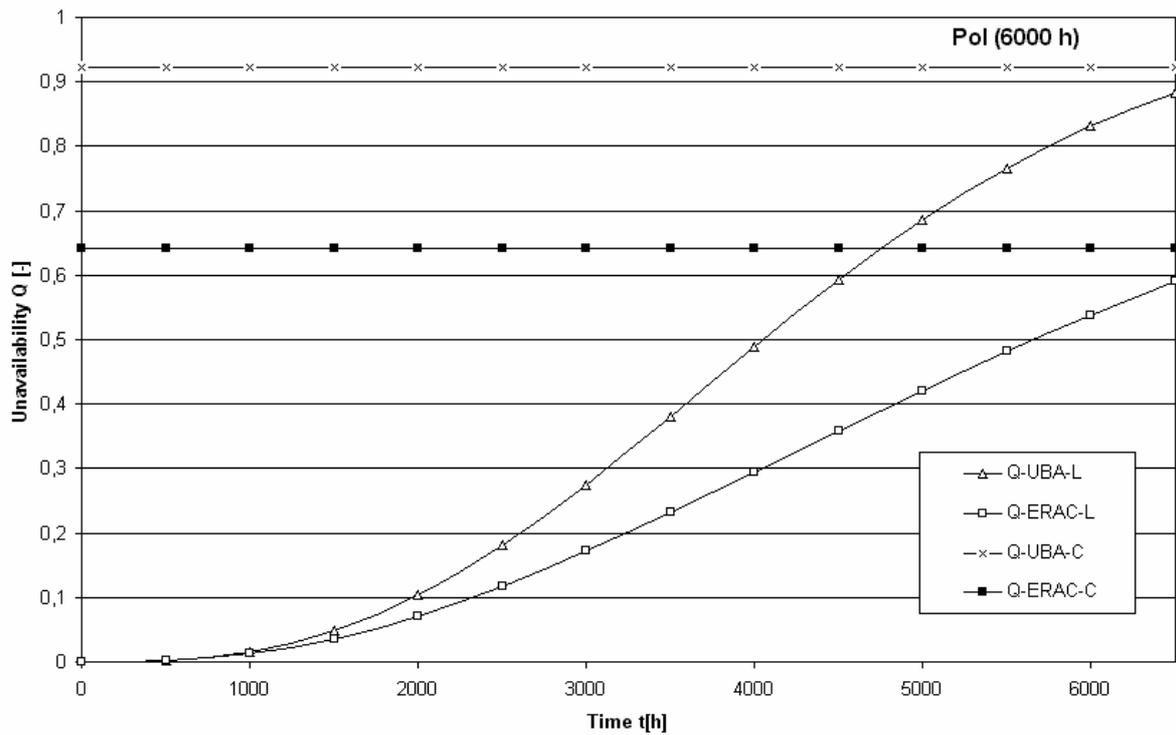
Fig. 11. The results of connected power plants simulation  $Q(t)$  for 6000 hours
