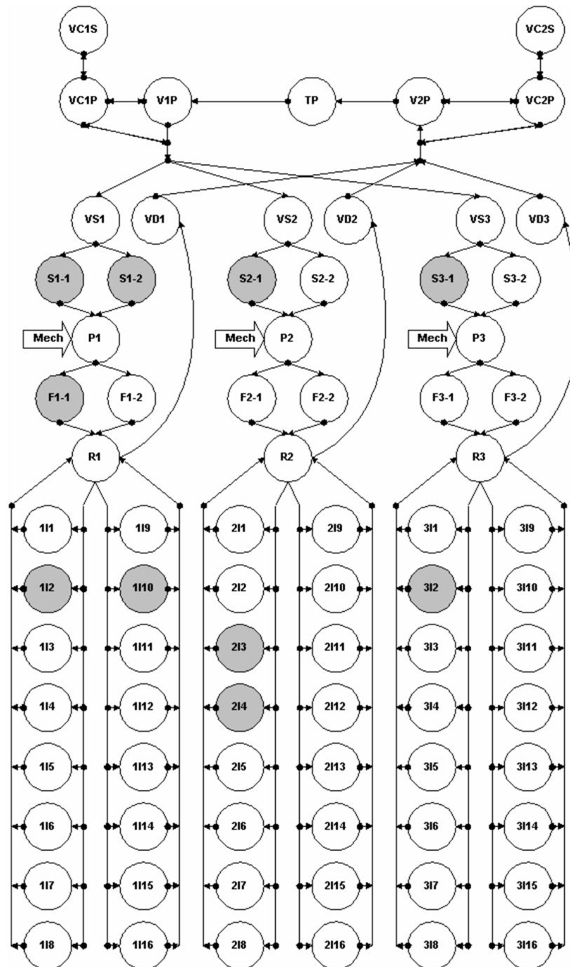
Fig. 4. Functional structure of energetic fluids flow in the port main engine room fuel supply system
