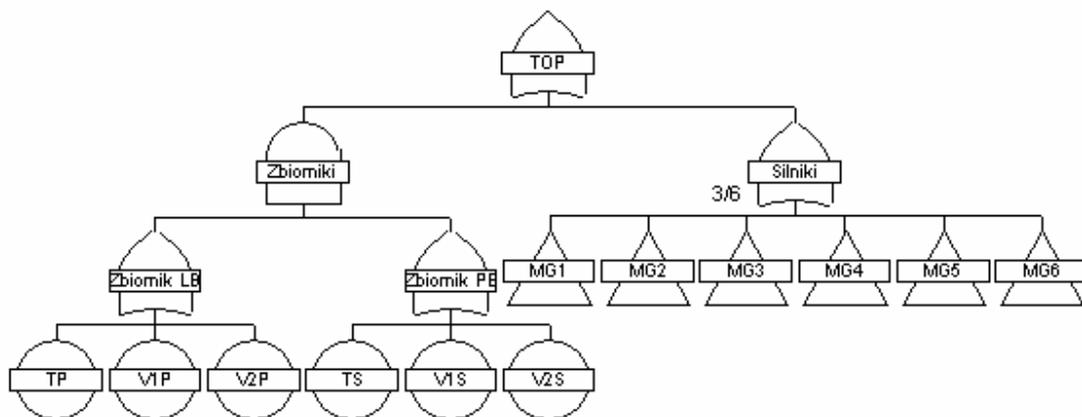
Fig.6. A fault tree for the fuel system of the generating set engines – valves separating power plants are open
