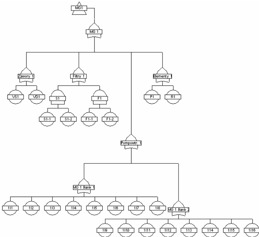
Fig. 8. A fault tree of the fuel system of an electric power plant engine (sub-tree of engine local installation – a case of MG1)
