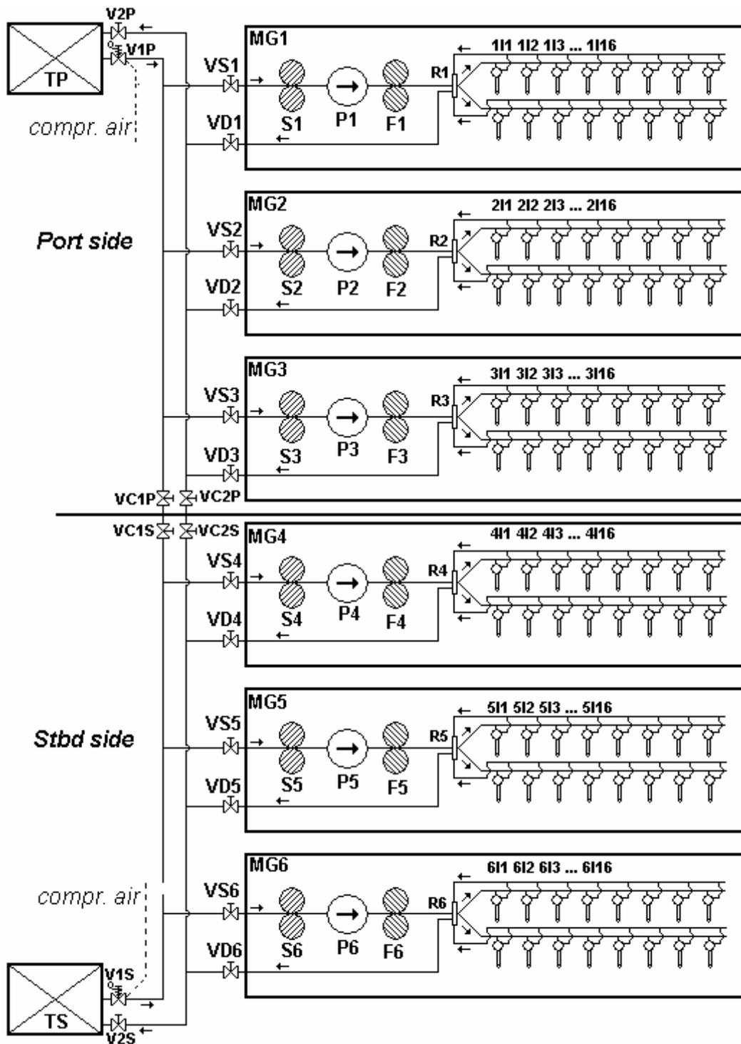
Fig. 3. The fuel system of the power-propulsion system
