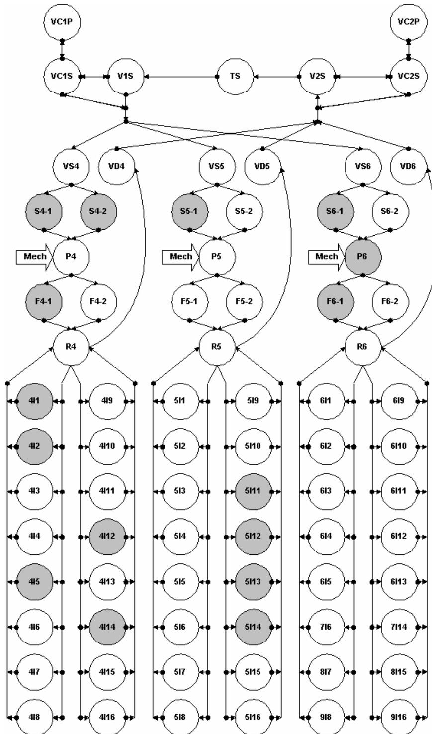
Fig. 5. Functional structure of energetic fluids flow in the starboard main engine room fuel supply system
