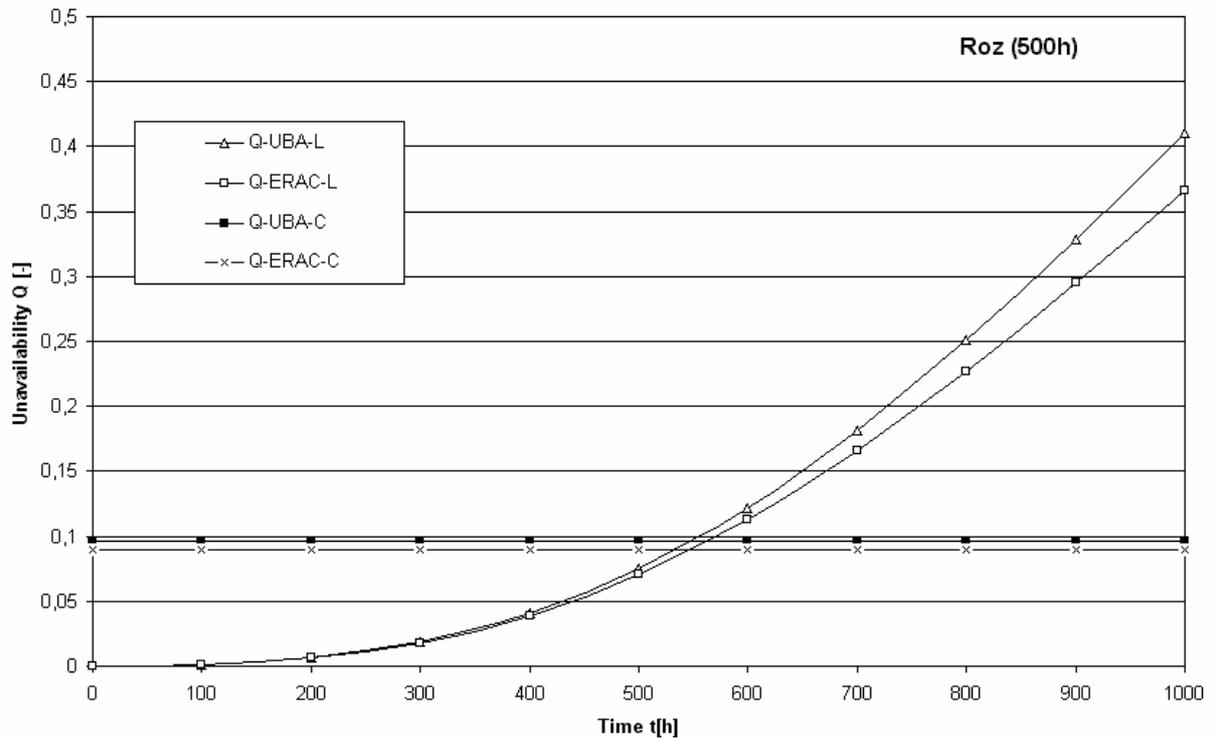
Fig. 10. The results of separated power plants simulation  $Q(t)$  for 500 hours
