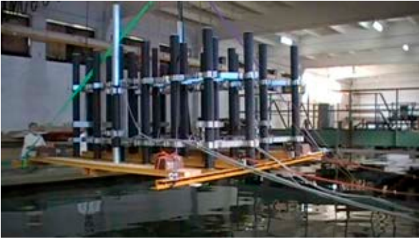
Figure 6. Testing the submarine breakwater prototype in the towing tank of the Ship Hydromechanics Division, Ship Design and Research Centre SA, Gdańsk (NCRD, 2010)
