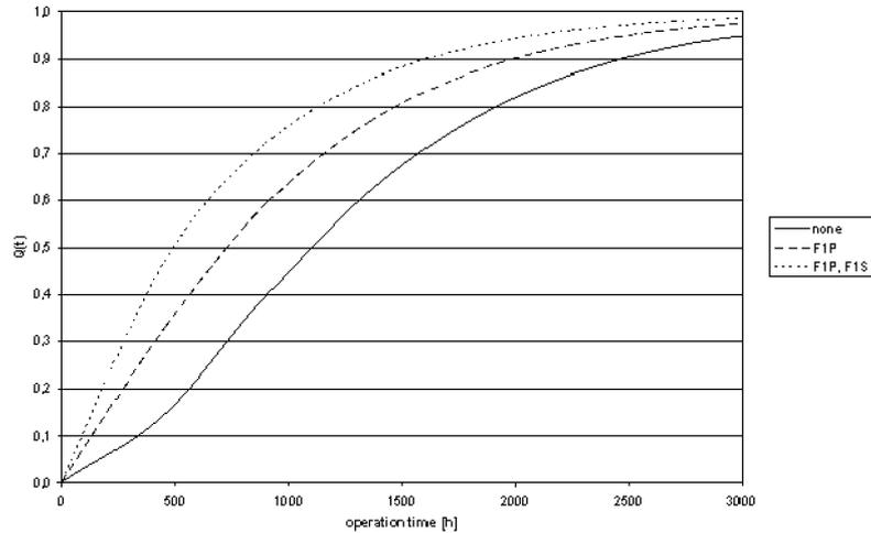
Fig. 3. Unavailability of the analyzed system for some strainers being out of operation at the start
