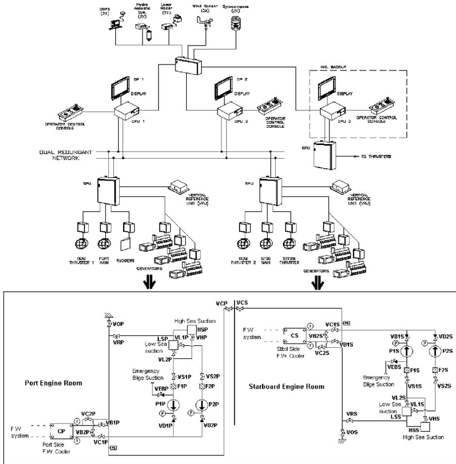
Fig. 1. Diagram of the analyzed sea water cooling system
