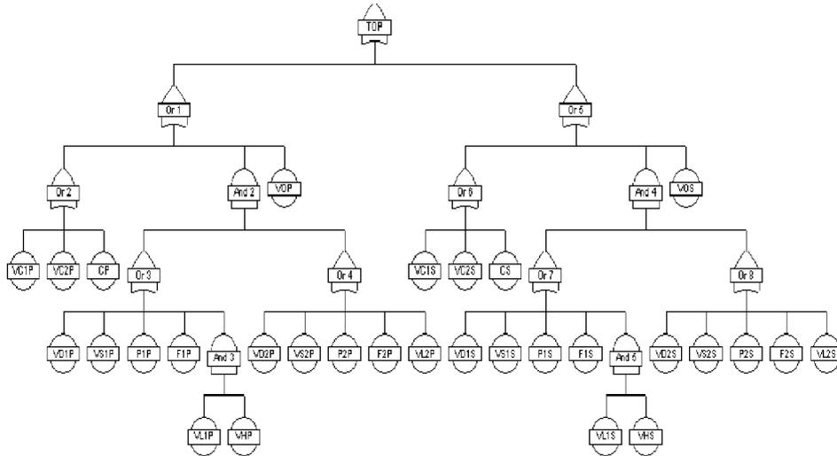
Fig. 2. Fault tree for the analyzed sea water cooling system for crossover valves in closed position
