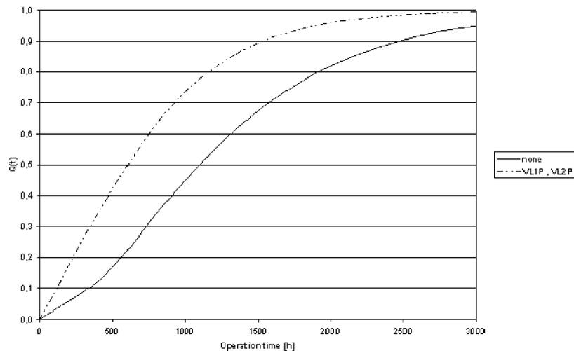
Fig. 4. Unavailability of the analyzed system for one sea chest being out of operation at the start
