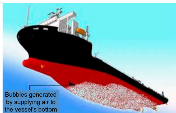
Figure 7. Air lubrication system for ships (Raunek, 2017)
