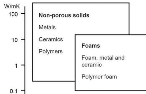
Fig. 4. The thermal conductivity of selected materials [13]
